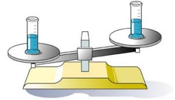
The **density**,  $d$ , of a substance is defined as the relationship between its mass and its volume.
